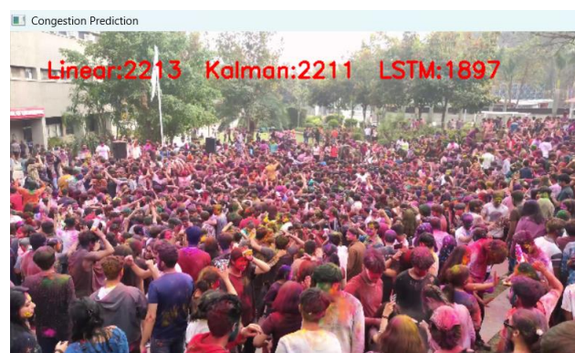
Figure. 4 demonstrates congestion prediction on a real-time basis on the Time-to-Congestion (TTC) of the Linear, Kalman, and LSTM models.
